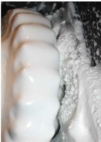
The grease distribution run at load step 12 showed that Klüberplex AG 11-461/462 adheres well to the tooth flanks and is not thrown off.
