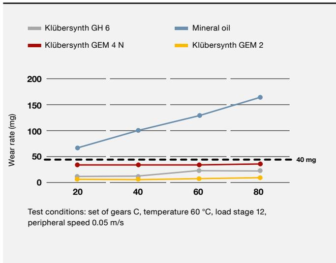
Test results obtained with high-performance gears oils made by Klüber Lubrication compared with mineral oil in FZG wear test
