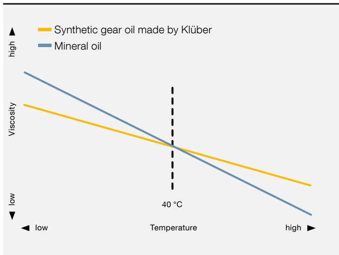
Klüber's high-performance gear oils show much better viscosity stability under varying operating conditions than mineral oils. A constant lubricant film can build up as the viscosity changes only slightly with temperature.
