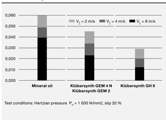
Comprehensive tests prove that synthetic gear oils have a much lower friction coefficient than mineral oils.
